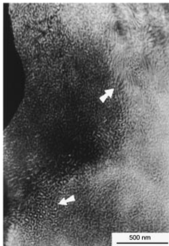
Figure 6. Transmission electron micrograph of S_{57}B_{27}C_{16} , which was compression molded and quenched in cold water (stained with OsO 4 ).
